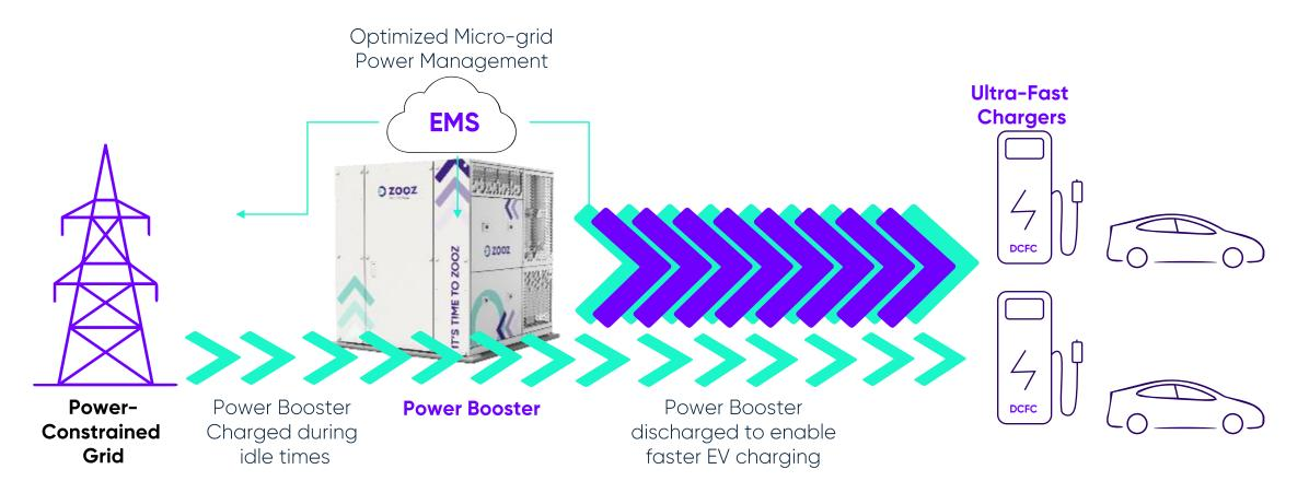
Enables Ultra-Fast Charging, even at power-limited grid
